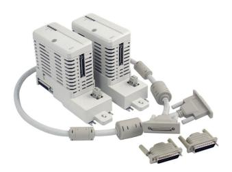
The BC810 unit consists of two basic parts: baseplate (TP857) and power supply/logic board. The baseplate is where the connectors to CEX-Bus and the external power reside. It is grounded to the DIN-rail through metal parts of the housing. The board also carries the external power voting diode and fuse. The power supply and logic board contains the +3.3 V converter, logic, drivers for CEX-Bus interconnection and the connector for interconnection cable.
