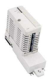
The DriveBus protocol is used to communicate with ABB Drives and ABB Special I/O units. DriveBus is connected to the controller via a C1858 communication interface unit. The DriveBus interface is used for communication between ABB Drives and AC 800M controller.
