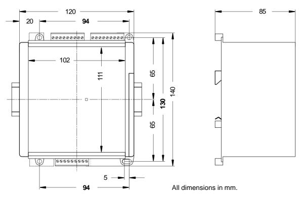
The depth of the module is 85 mm. If a DIN rail is used, the installation depth must be increased by the dimension of the rail.
