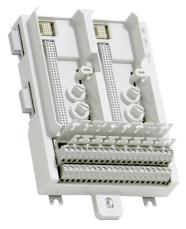
The TU844 MTU can have up to 8 I/O channels and 2+2 process voltage connections. Each channel has two I/O connections and one ZP connection. Input signals are connected via individual shunt sticks, TY801. The shunt stick is used to choose between voltage and current input. The maximum rated voltage is 50 V and maximum rated current is 2 A per channel.
